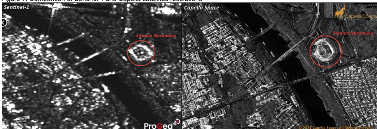
Figure 7. Comparison of Sentinel 1 and Capella satellites resolutions
